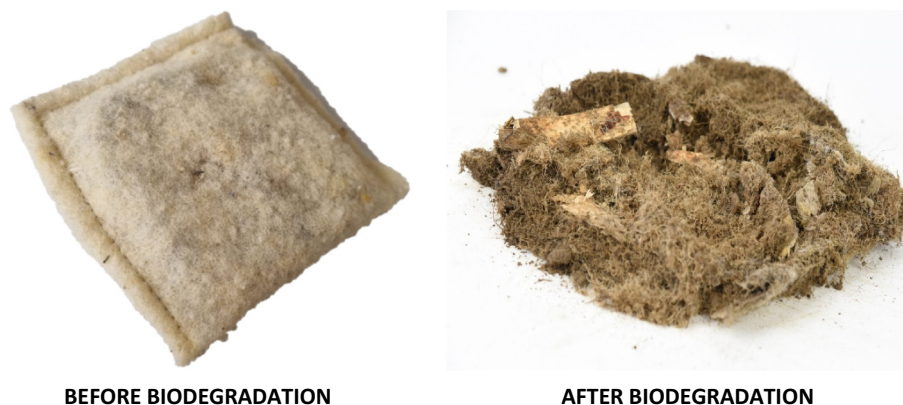
Fig. 11. Overview of the condition of needle-punched nonwovens before and after biodegradation (1 year).
