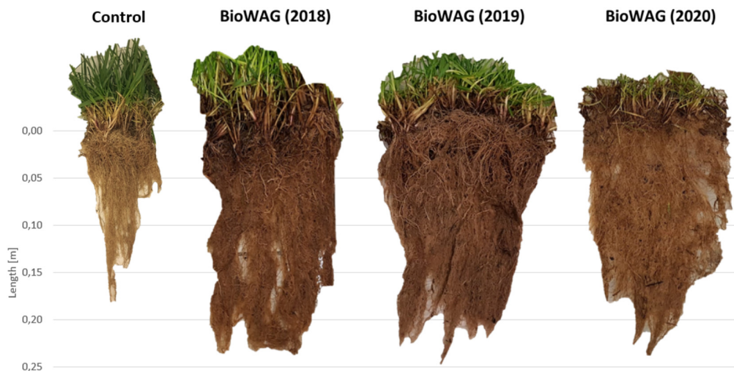
Fig. 6. Development of the root system on a control site and a site with BioWAG in the years 2018–2020.
