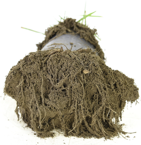
Fig. 6. Grass root system that formed on needle-punched nonwoven, 100% wool (BB).
