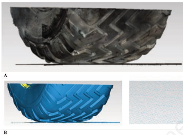
Figure 4. A) A spatial image of a tire profile consisting of a point cloud. B) View of the created triangle mesh prepared for cross-sectional processing (left), the effect of zooming triangle mesh (right).
