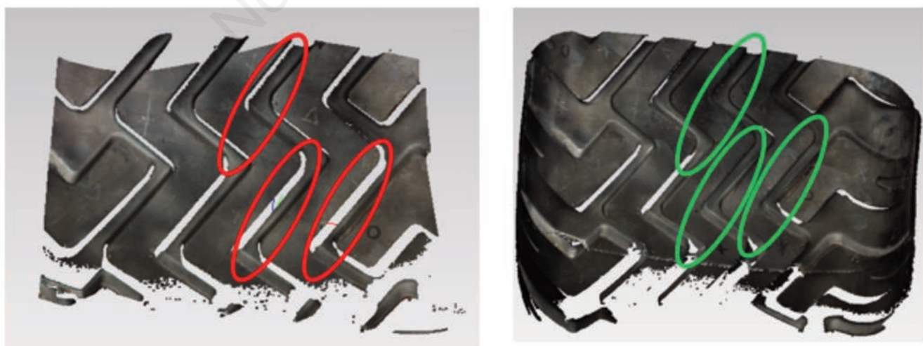
Figure 3. Tread scanning effects: the effect with scanner location points evenly spaced (left), the effect with scanner location points unevenly spaced (right).
