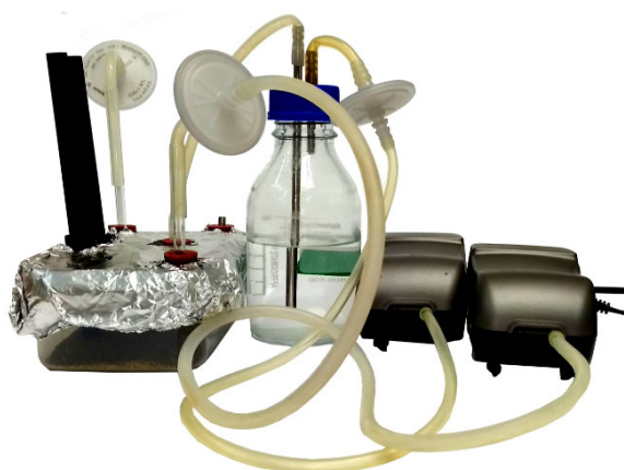
Figure S14. A bioreactor vessel with graphite electrodes, a vessel with water, air and water pumps.
