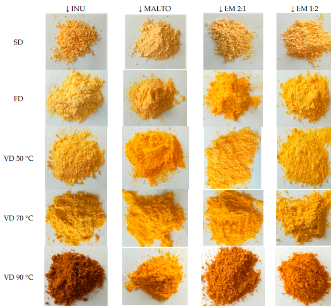
Figure 1. Color of sea buckthorn juice powders modulated by drying methods and carrier agents. SD, spray drying; FD, freeze drying; VD, vacuum drying; INU, inulin; MALTO, maltodextrin; I:M, inulin:maltodextrin.
